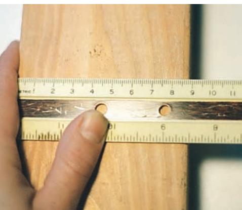
FIGURE 1-2 Measuring the width of a board with a centimeter ruler. The uncertainty is about \pm 1 mm.
